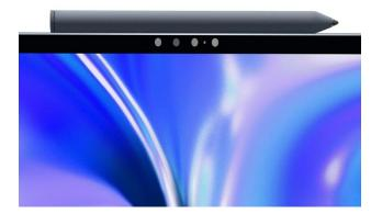
The XPS comes with a Bluetooth Stylus, which magnetically "docks" on the top edge of the system. This also charges the pen.
