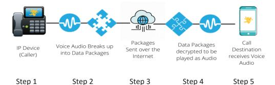
Modern VoIP technology allows voice data to be transmitted in a digital format on IP networks, allowing for cost-effective and flexible communication. It allows voice data to be sent to a variety of recipient devices and is not constrained to using traditional telephone lines.
